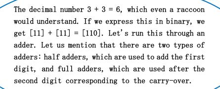
Additive circuits for arithmetic circuits (half and full adders)
